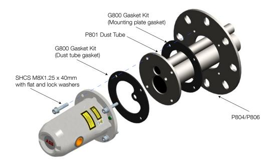
Figure 4-8. Mounting Plate Assembly
